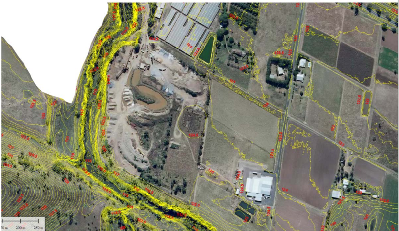
Plate 3: Reconstructed topographic plan of Batching Plant Site superimposed on LiDAR survey
